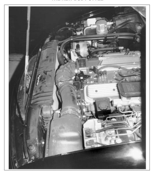
This shows how tight it is between the engine and radiator. The air cleaner ducting is extremely close to the radiator, even though the  $90^{\circ}$  rubber elbow attached to the throttle-body (from a 94-97 Camaro LT1) was trimmed to gain about 3/4" clearance. The air cleaner box is from a 1994-1996 Caprice.
